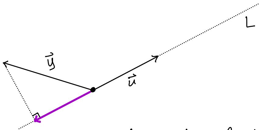
orthogonal projection of  $\vec{y}$  onto  $\vec{u}$
